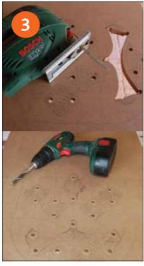
Move the panel down so that the top is centred between the two work benches and clamp securely. Use a drill/driver and 10mm wood bit to drill out holes in the drawn designs. Insert the blade of the jigsaw into the holes to cut out the designs. Cut slowly and gently guide the jigsaw around curves.
