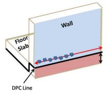
Drill Holes are spaced 100mm apart. Drilling & Injection will be done 1-brick height above the DPC line i.e on the red line in the diagram.
